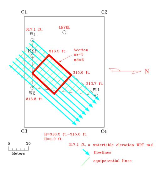
Figure 3. Mercer Soccer Field With Flowlines and Equipotential Lines
