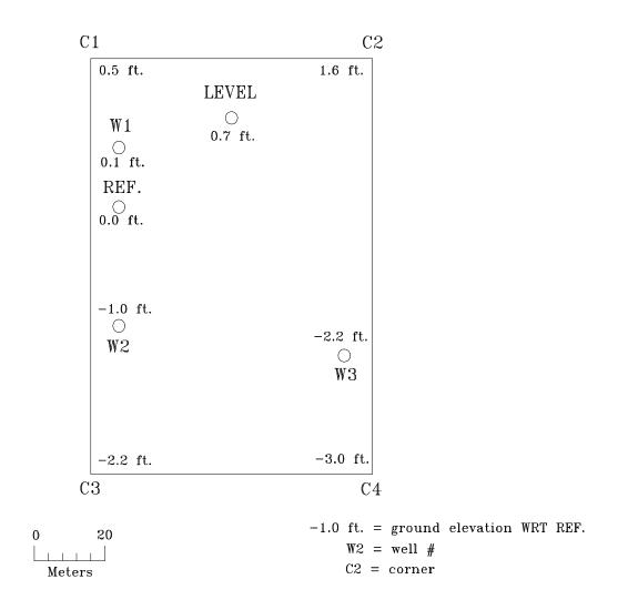
Figure 2. Mercer Soccer Field With Ground Elevations
