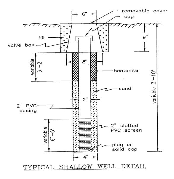
Figure 1. Typical Shallow Well Detail
