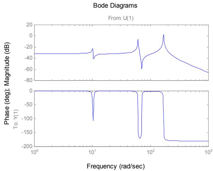
Figure 5: Bode Plot of Smart Flexible Beam System
