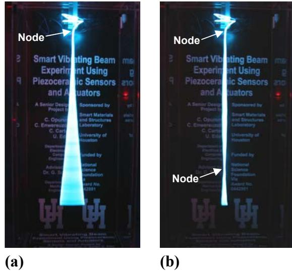
Figure 4: (a) First and (b) Second Mode Operation of Smart Flexible Beam
