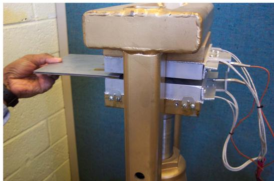
Figure 3: MEA Going into Hot Press.
