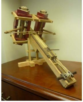
Figure 1 The form of the ballista that is described by Heron and Philon.
