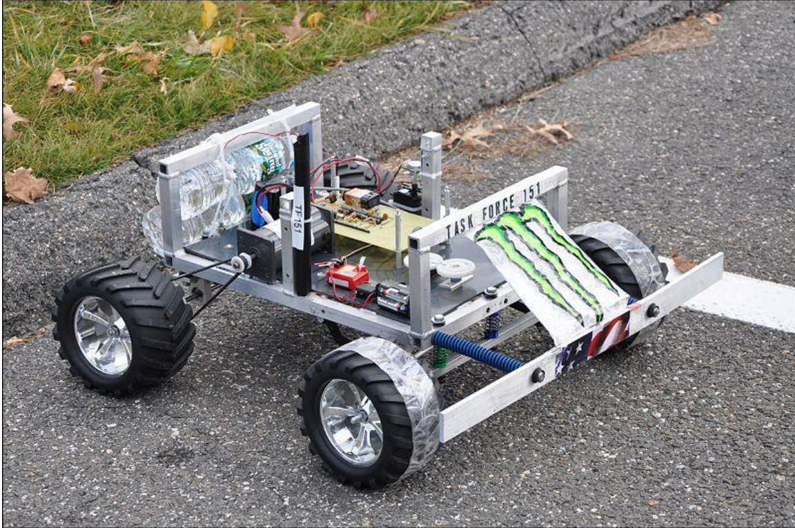
Figure 5: The monster truck vehicle prototype. Tape was used to reduce friction and allow the steering servo to turn the wheels.
