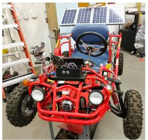
Figure 1. The Smart Kart front view, with visible ultrasonic sensors, robotic arm, steering assembly, and 40W solar panel array
