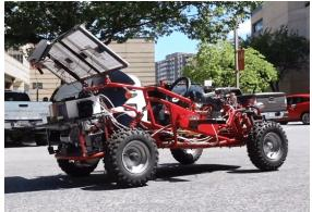
Figure 2. The Smart Kart side view, with visible battery array, 1.8kW motor, and solar charge controller
