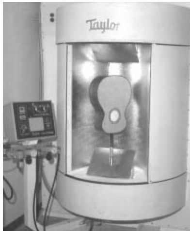
Figure 1: Ultraviolet curing chamber at Taylor Guitars, El Cajon, CA 9 .
