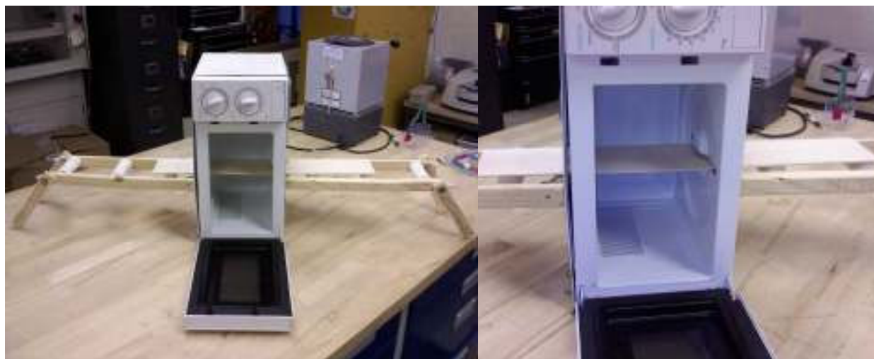
Figure 3: Modified home-model microwave for multimode microwave curing of wood planks.
