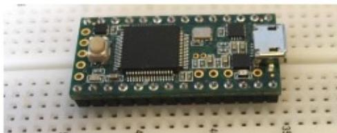
Figure 4: Teensy 3.2 board placement in a breadboard.
