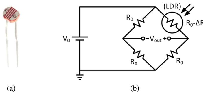
Figure 3: (a) light-dependent-resistor (LDR) (b) Wheatstone bridge light sensor circuit
