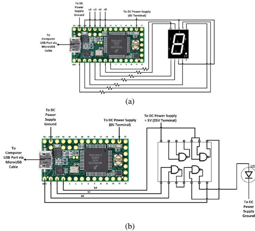
Figure 5: (a) Analog to binary-coded-decimal circuit (b) Threshold detector circuit using Teensy board's ADC and a NAND IC
