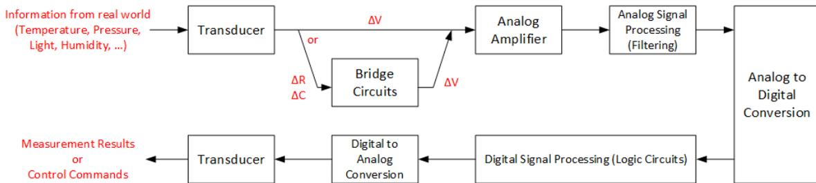
Figure 1: The general block diagram of an instrumentation system
