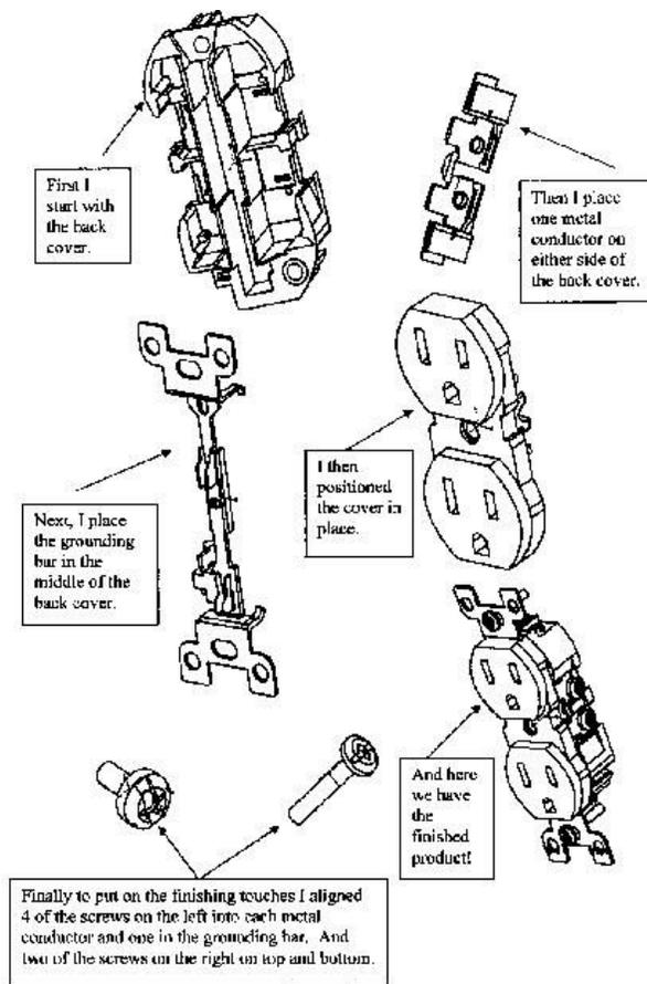
Fig 1. Electric Receptacle Project
