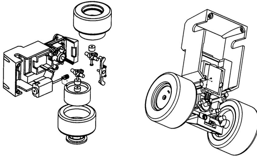
Fig 2. Toy Car Steering Mechanism Project
