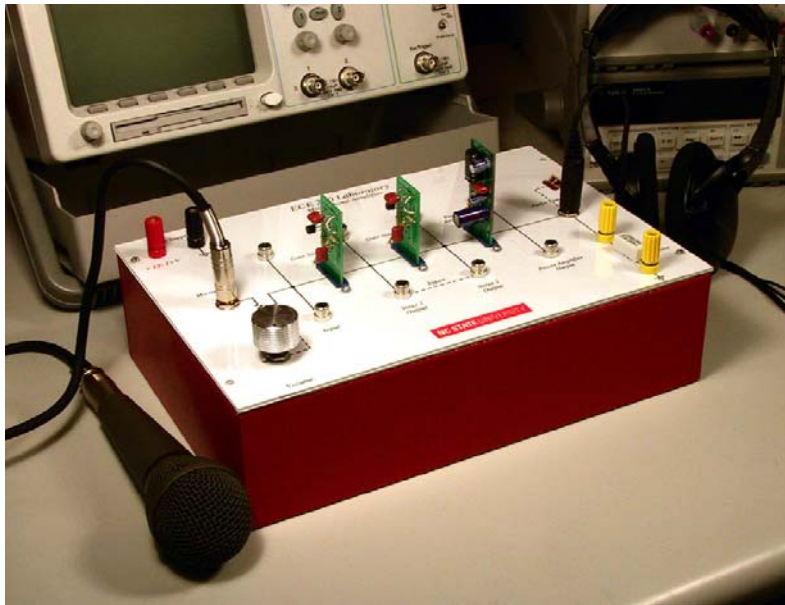
Figure 6 The experiment box used for Experiment 6 is a three-stage microphone amplifier consisting of two common-source MOSFET amplifier stages and a unity gain power amplifier stage. Students can easily monitor the signals at different stages of the amplifier using the connectors on the front panel of the experiment box.
