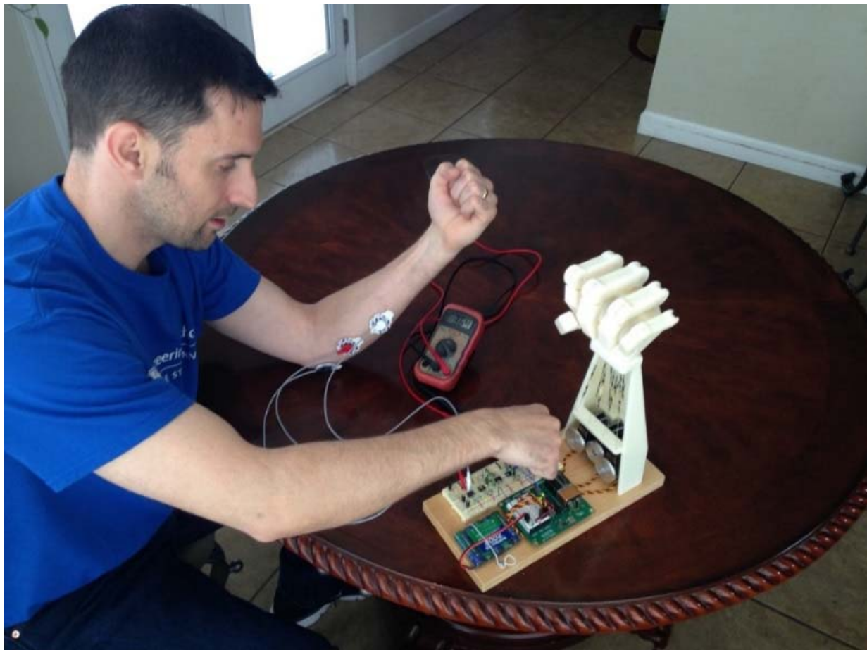
Figure 11: Calibration of the bionic hand
