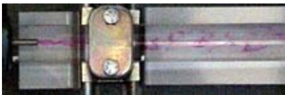
Figure 8. Flow streams inside empty tube at various Reynolds numbers
