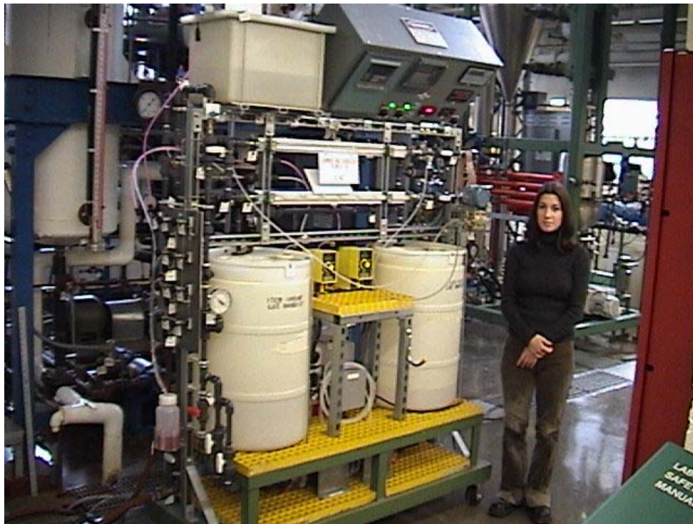
Figure 3. Laminar/Turbulent Flow Demonstration Module "Proceedings of the 2003 American Society for Engineering Education Annual Conference & Exposition Copyright © 2003, American Society for Engineering Education"
