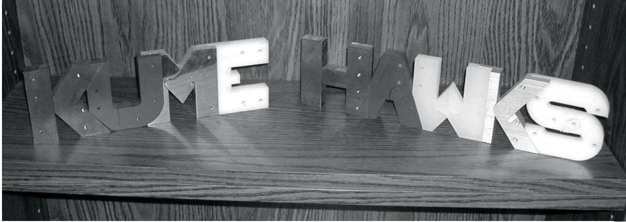
Figure 1. “KUME” and “HAWKS” letters machined using a three-axis CNC vertical mill.
