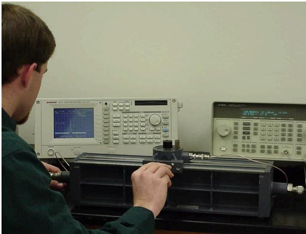
Figure 4: Slotted-Line and Signal Generator
