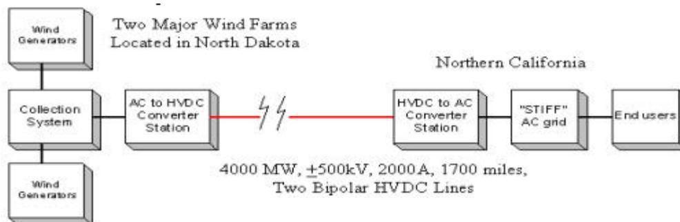
Figure 10. A functional block diagram of proposed 4,000 MW,  $\pm 500$  kV, 2,000A, 1,700 miles, Two Bipolar HVDC System.
