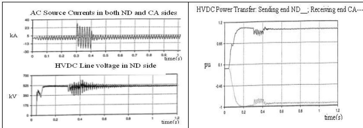
Figure 11. AC current waveforms in both ND and CA sides and DC line voltage during the fault and sending and receiving end DC power waveforms
