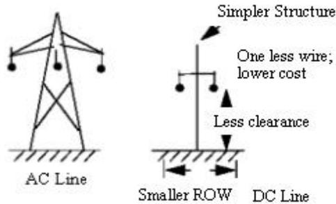
Figure 1. AC and DC Transmission Towers
