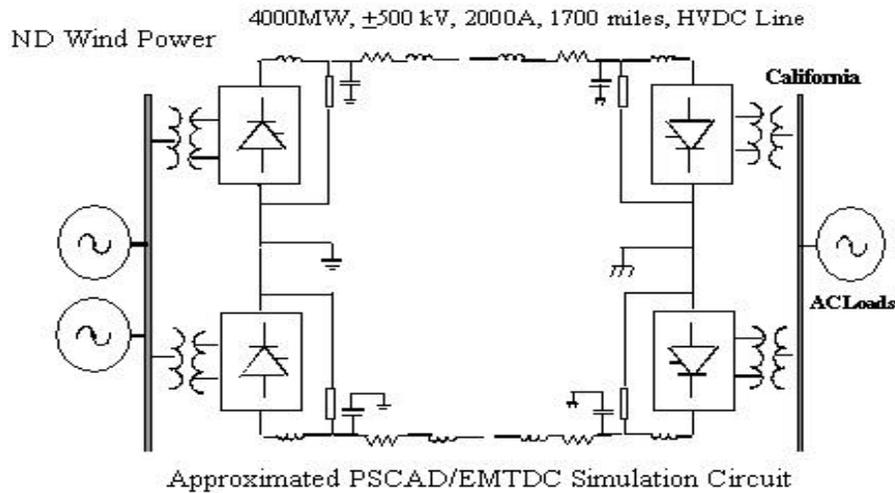
Figure 9. Proposed Bipolar HVDC System.
