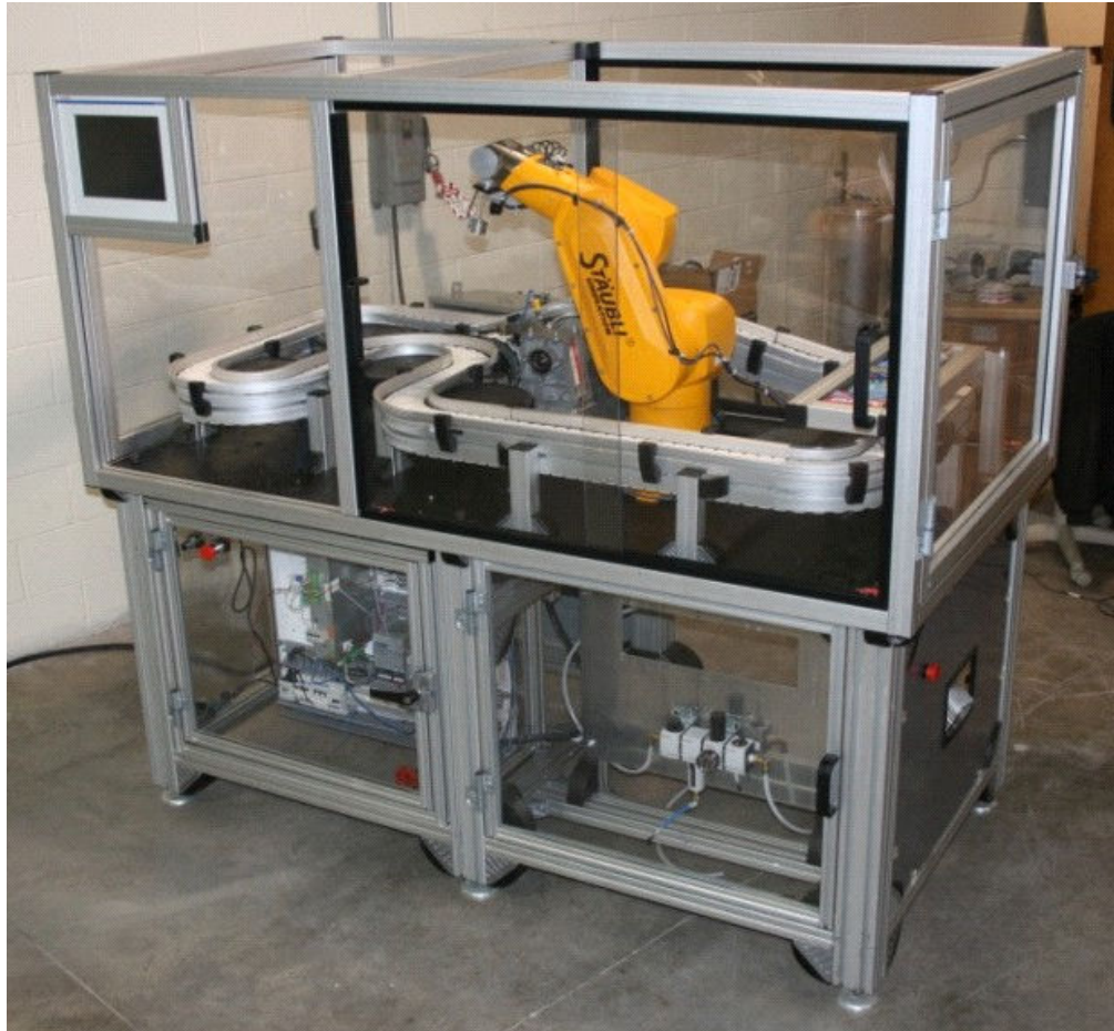
Figure 1: Portable robotic workcell integrating a robot manipulator with vision and conveyor systems.
