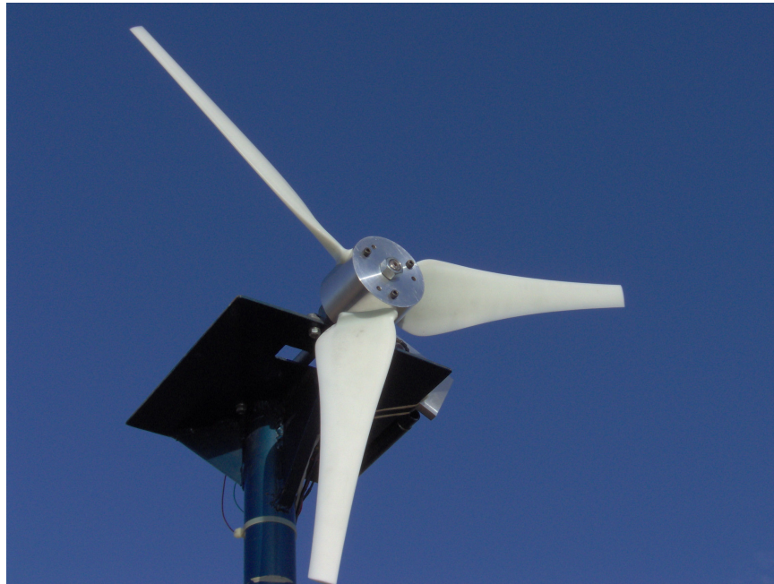
Figure 1: A student-designed horizontal-axis wind-turbine rotor mounted on the teststand
