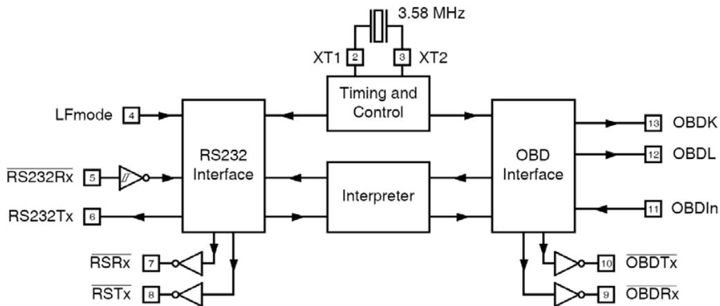
Figure 1. OBD to RS232 Interpreter Circuit
