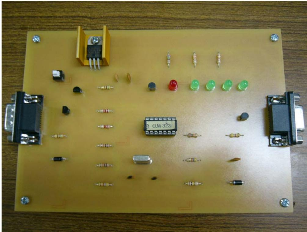
Figure 2. OBD to RS232 interpreter printed circuit board
