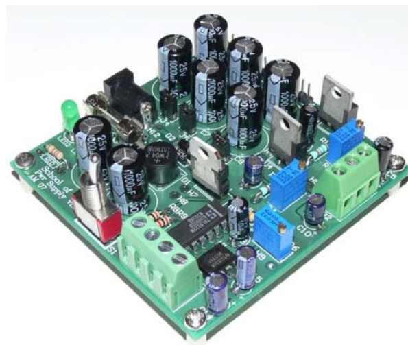
Figure 2. Completed power supply
