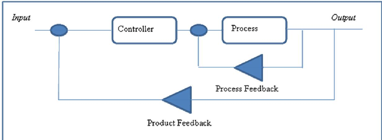
Figure 2. A production control model with warranty.
