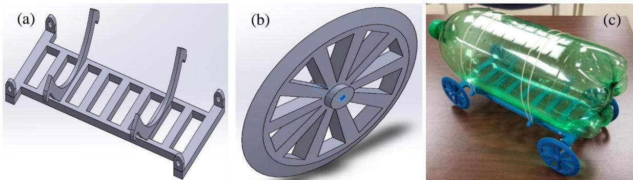
Figure 2: 3-dimensional CAD design of a modified (a) chassis, (b) wheel and (c) re-designed assembly of 3D printed chassis and wheels.
