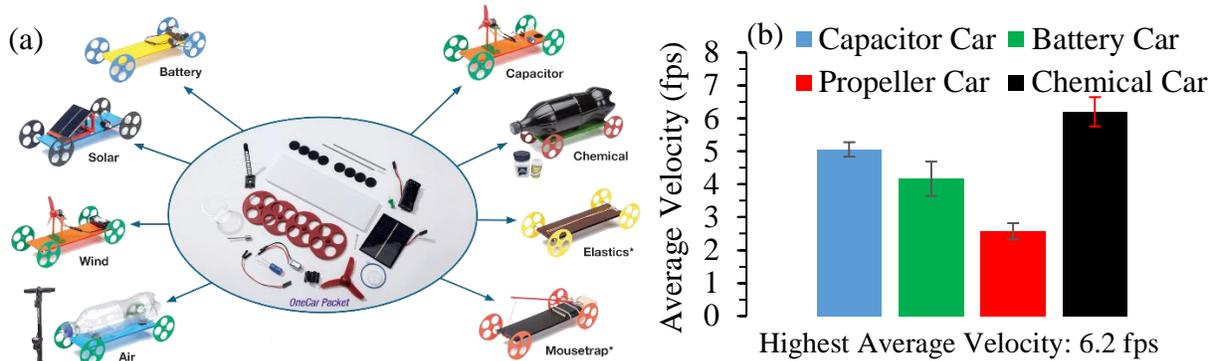
Figure 1: (a) Image of the OneCar™ STEM kit displaying assembled cars with the respective eight energy sources, and other components. (b) Results of initial product performance displaying average velocity (in feet per second) for the capacitor, battery, propeller and chemical energy sources.
