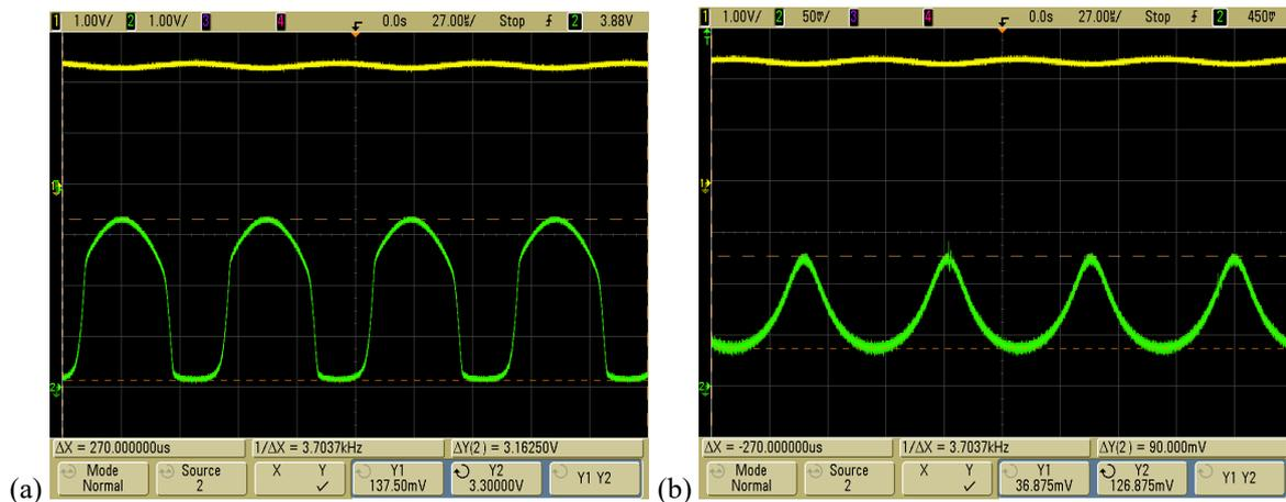
**Fig. 8** Common source amplifier working in linear region with, (a) 1KΩ load resistor using switch S1 and, (b) 2.2KΩ load resistor using switch S2. The yellow waveform is small signal input whereas green waveform is the amplifier output.
