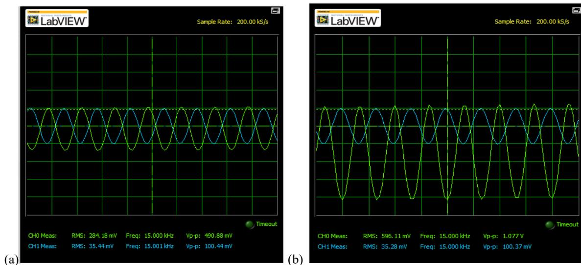
**Fig. 9** Differential amplifier working in saturation region with, (a) 1KΩ load resistor using switch S1 and, (b) 2.2KΩ load resistor using switch S2. Blue is the input and green is the output waveform.
