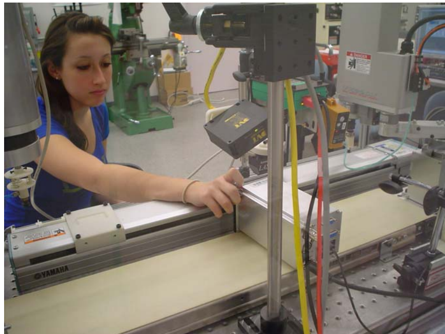
Figure 9: Student conducting traveling distance testing and calibrating robotic accuracy
