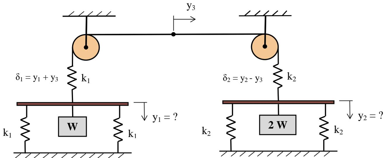
Figure 4 – Problem (5) – Adding the displacement variable “ $y_3$ ,” needed for describing upper spring deflections  $\delta_1$  &  $\delta_2$
