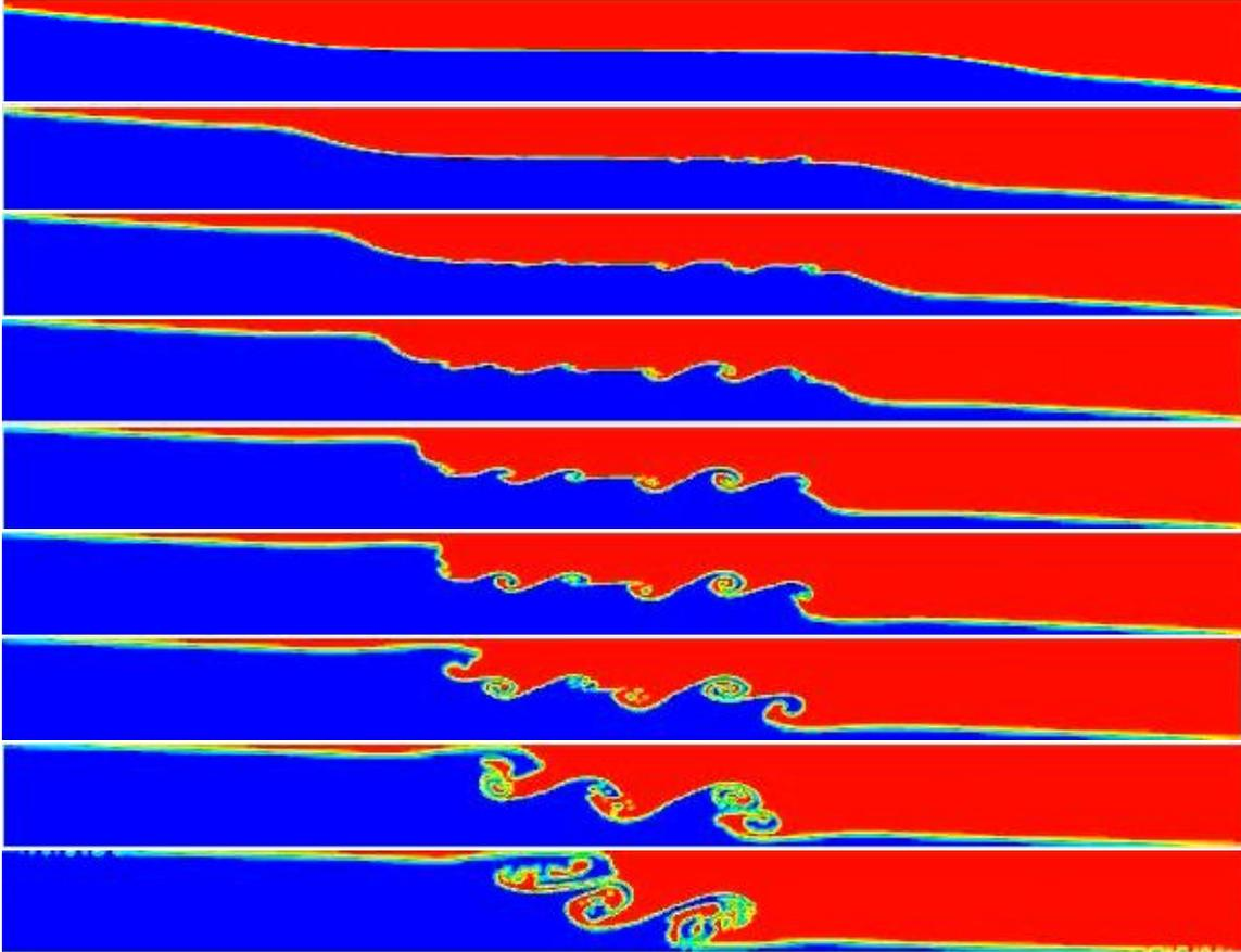
**Figure 5b).** Contour of volume fraction for water at  $t = 0.0, 1.4, 2.6, 3.5, 4.3, 4.7, 5.0, 5.2, 5.4, 5.6, 6.0$  and  $6.5$  s.
