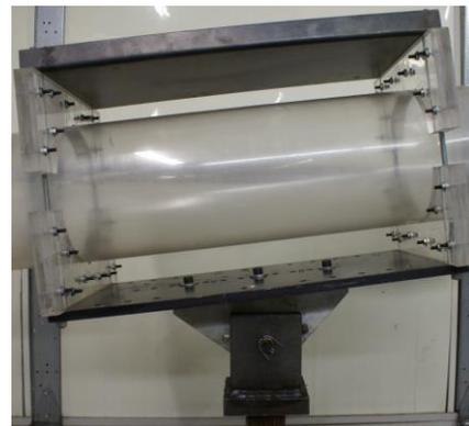
**Figure 2d).** Support structure for tube
