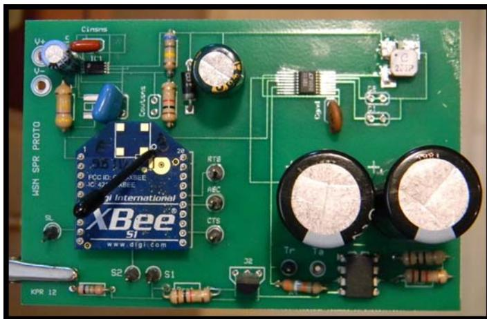
Figure 4 Energy harvesting circuit
