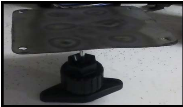
Figure 7 Pivoting solar panel mount.
