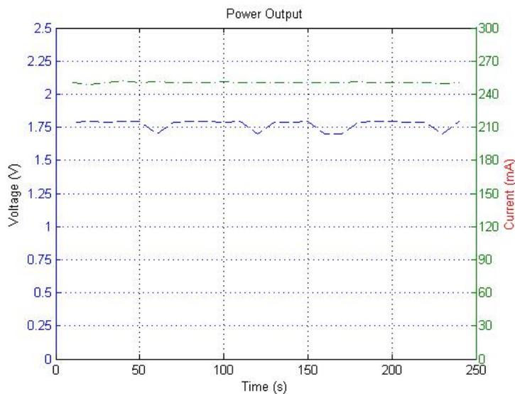
Figure 6 Waveforms showing PV voltage and PV current
