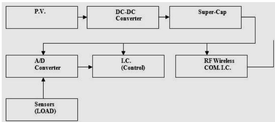
Figure 3 Harvester block diagram
