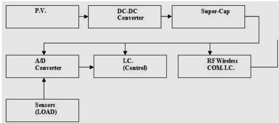
Figure 3 Harvester block diagram
