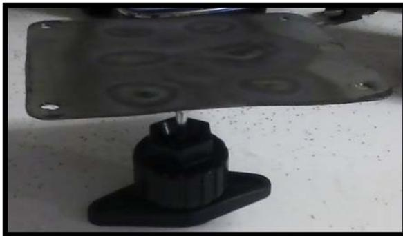
Figure 7 Pivoting solar panel mount.
