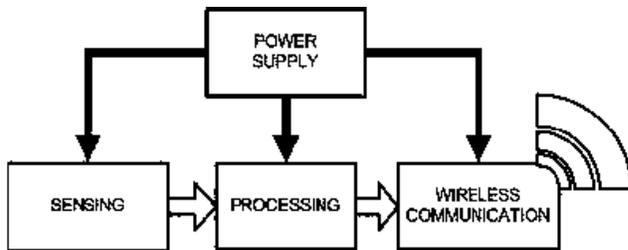
Figure 1. Block diagram of a sensor node
