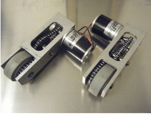
Fig 4 DC Motors and Drive Trains
