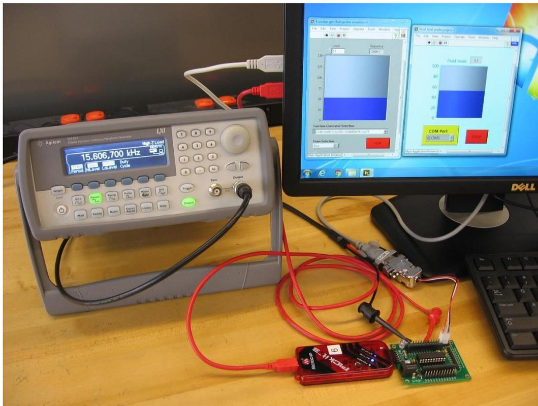
Figure 9. Hardware In the Loop testing setup
