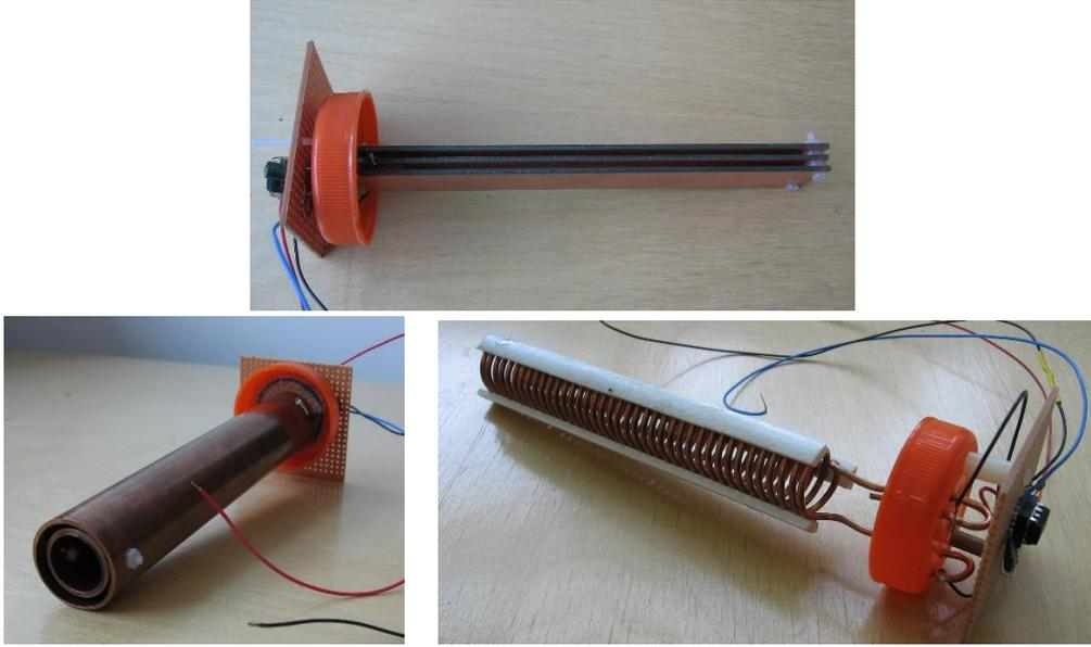
Figure 3. Examples of Student Capacitive Fluid Probe Designs
