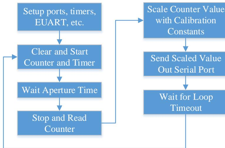
Figure 7. Flowchart of microcontroller code
