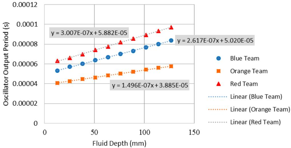
Figure 6. Sample of probe data manipulated to find desired calibration constants
