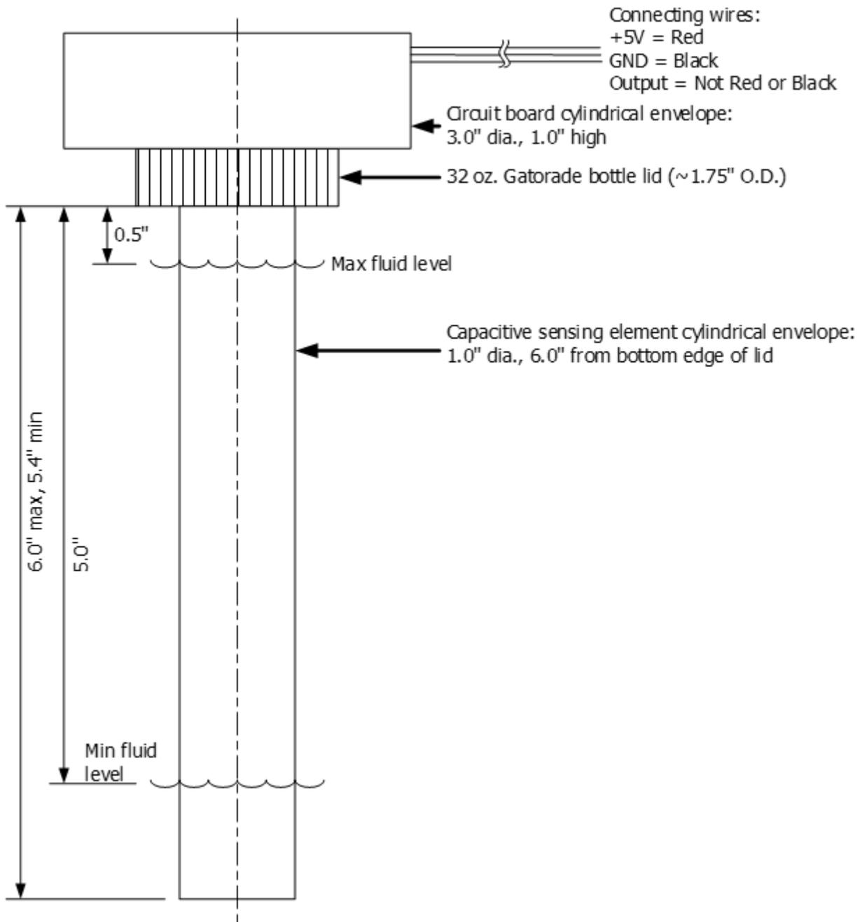
Figure 1. Capacitive Fluid Level Probe Specification Diagram
