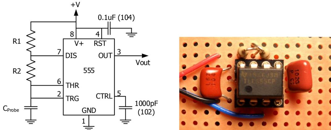
Figure 2. 555 Timer Oscillator Circuit Schematic and Suggested Circuit Board Layout
