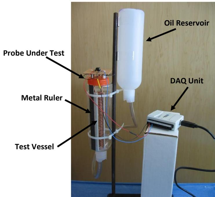
Figure 4. Probe test and calibration setup
