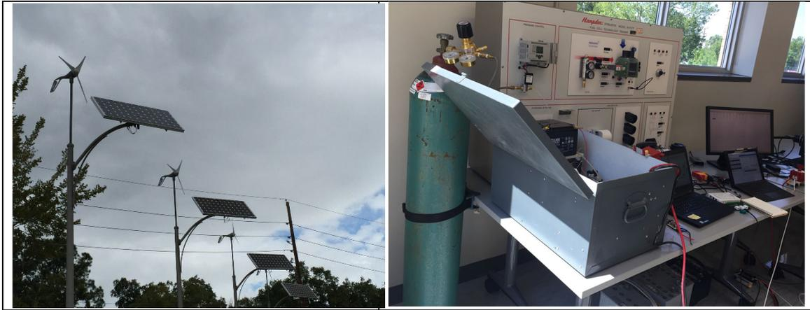
Figure 2. Solar PV, wind turbine, and hydrogen fuel cell power system that establishes a microgrid to smart grid test bench.
