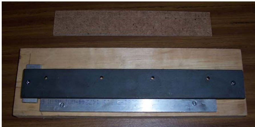
Figure 2. Drilling tool guide with masonite strip
