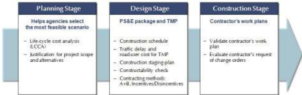
Figure 3. Use of CA4PRS throughout project life cycle
