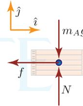
**Material Models** Since we want the *minimum* coefficient of static friction between the crate and truck required for no sliding, that means that slip must be impending and so
