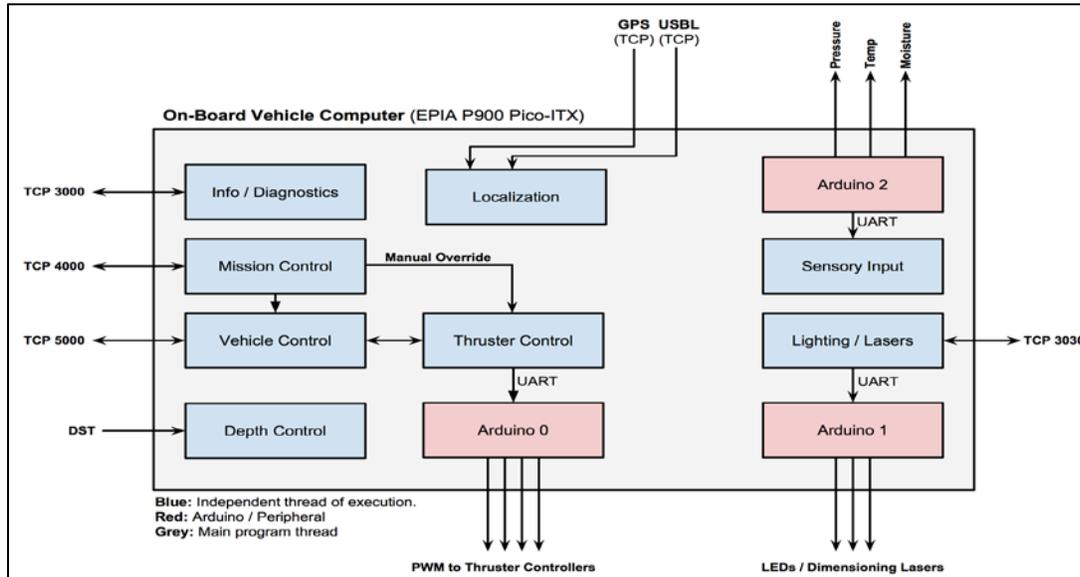
Figure 5: Vehicle Control Software
