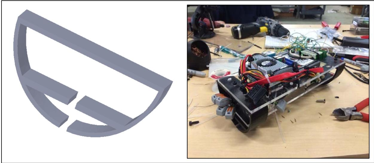
Figure 10: Electronics assembly with 3D printed support frame
