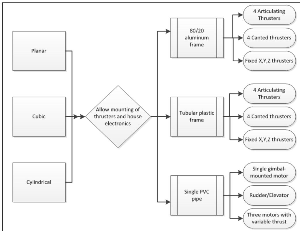
Figure 3: Concept Tree for Vehicle Form
