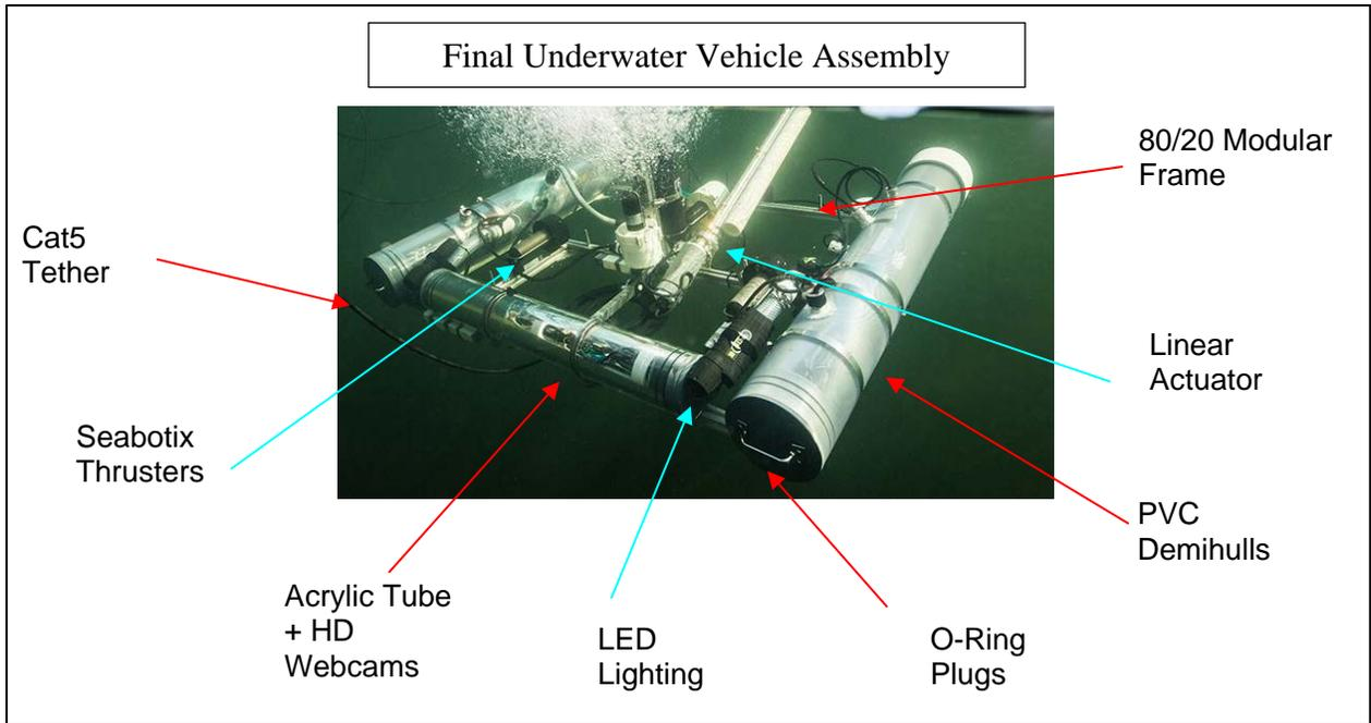
Figure 11: Final Vehicle Assembly
