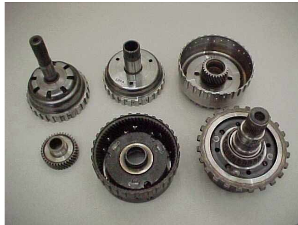
Figure 3. Working Demo of Planetary Sets and Input/Reaction Splines. Working Demo is Disassembled into Six Pieces at Right.
