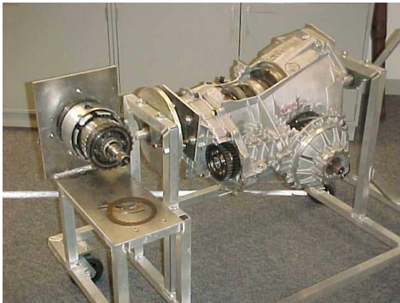
Figure 2. Portable Static Cutaway Display. Removable Working Demo of Gear/Spline Assembly is Shown at Left Mounted on Actual Input Shaft.
