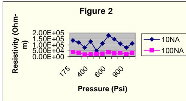
Figure 2: Resistivity Of Electrolyte Matrix Versus Fabrication Pressure At Various Nano-Amps.
