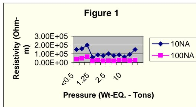
Figure 1: Resistivity Of Electrolyte Matrix Versus Fabrication Pressure At Various Nano-Amps.
