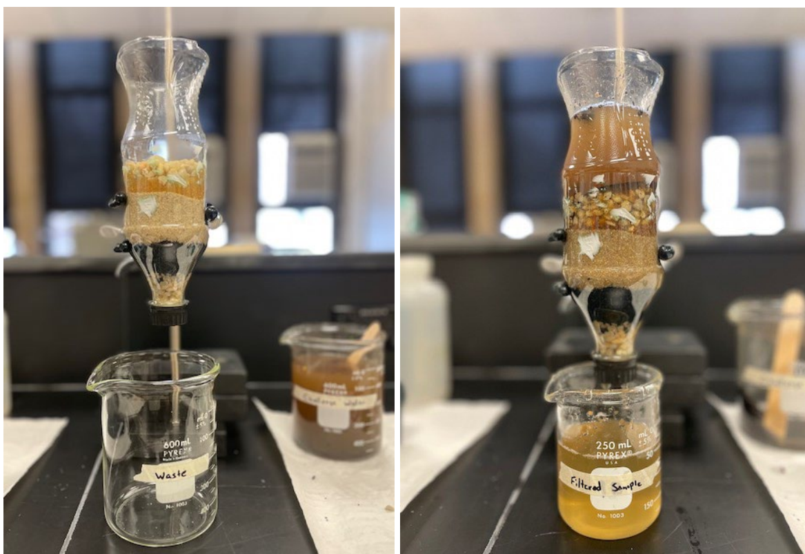
Figure 5a. Example of a student designed filter and the function of the filter.
