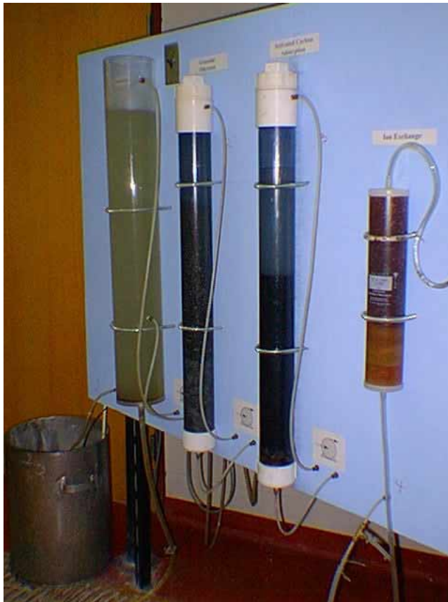
Figure 2. Photograph Showing Ion Exchange Color Bands
