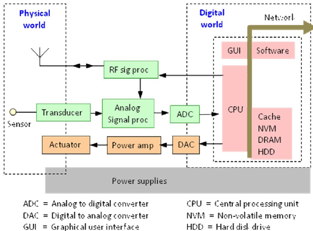
Figure 2. Generic representation of an electronic system
