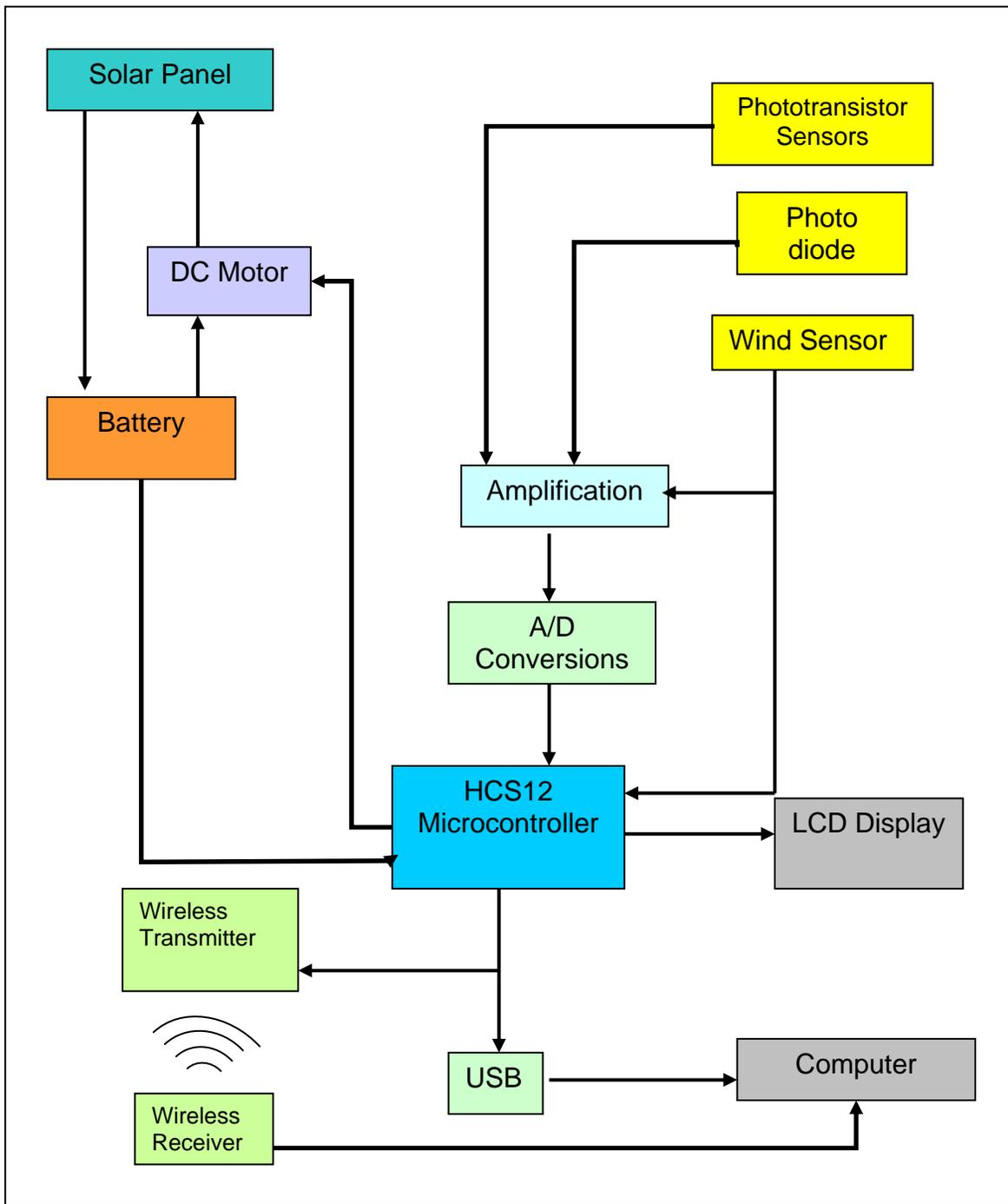
Figure 1: Solar Insolation Measurement System Block Diagram
