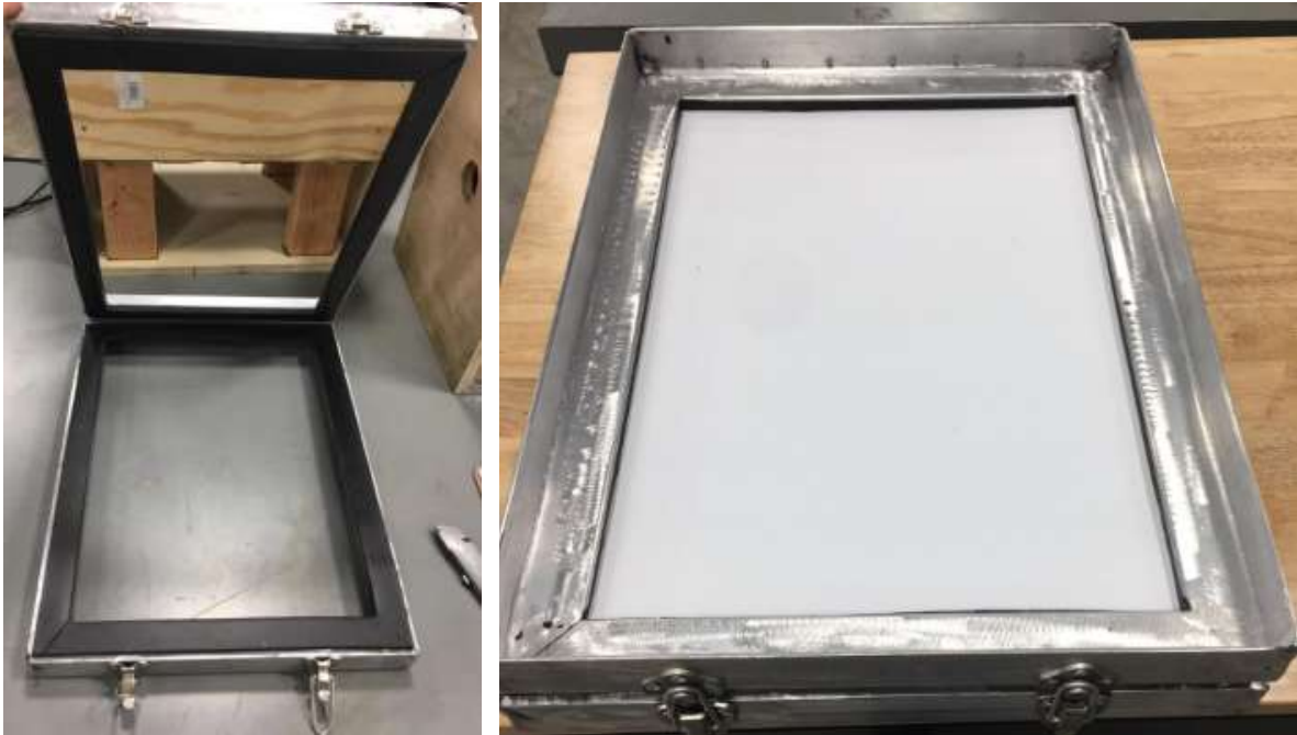
Figure 4a) Open and locked aluminum frame for plastic sheet
