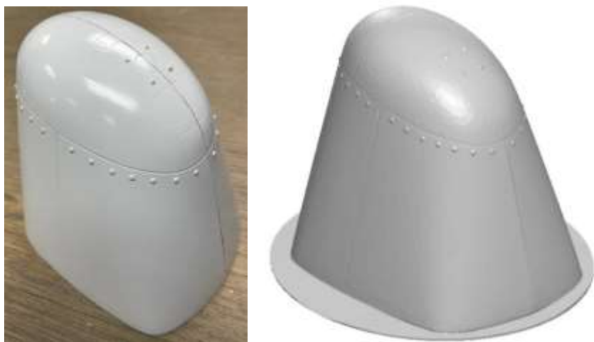
Figure 2c) Cowl made of fiberglass and shown as a 3D scanned model
