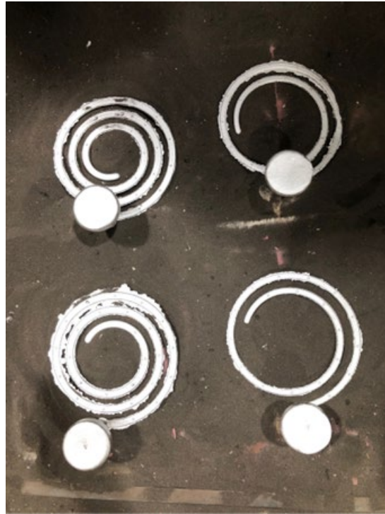
Figure 4. Fluidity spirals produced by pouring A356 aluminum into 3D printed sand molds using different pour temperatures and alloy chemical compositions.
