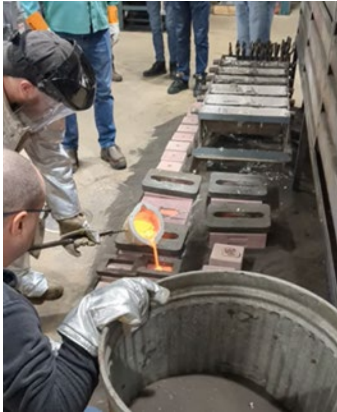
Figure 1. A METAL level one bootcamp participant pouring A356 (i.e., an aluminium casting alloy) into a 3D printed sand mold.
