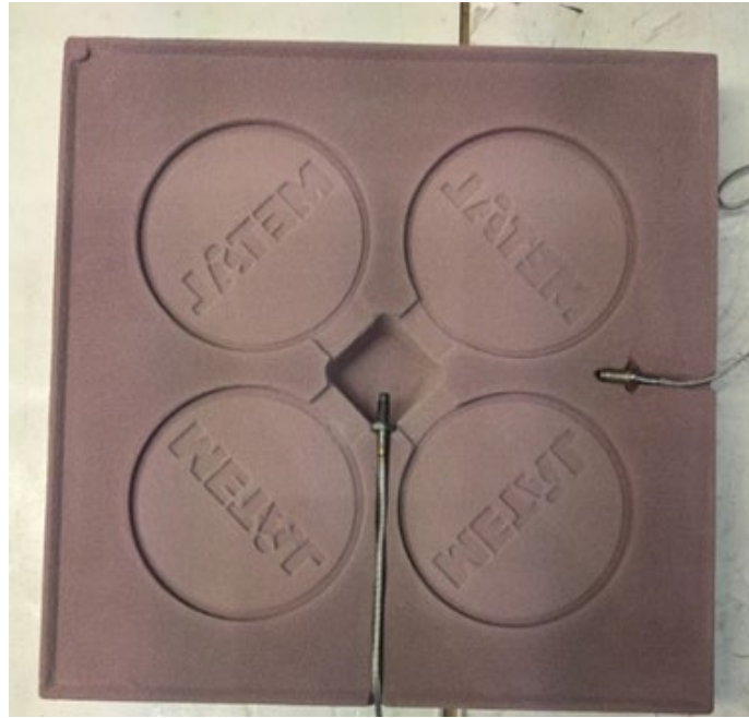
Figure 3. An instrumented sand mold, manufactured by 3D binder jet sand printing, used to cast the METAL medallion.
