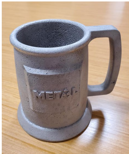
Figure 5. A356 aluminum stein mug produced by lost foam casting (left). A356 aluminum ACE air engine base produced by sand casting (right).
