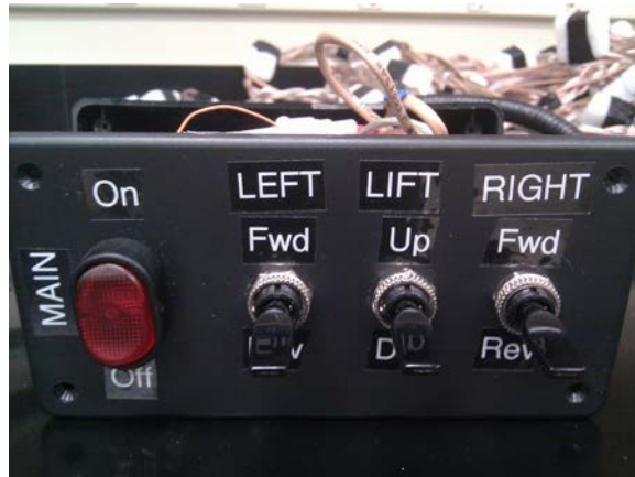
Figure 6. Control box front panel.
