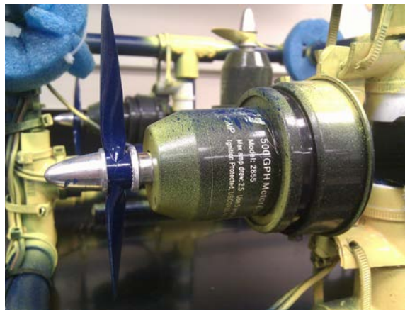
Figure 3. Horizontal thruster and mounting brackets.
