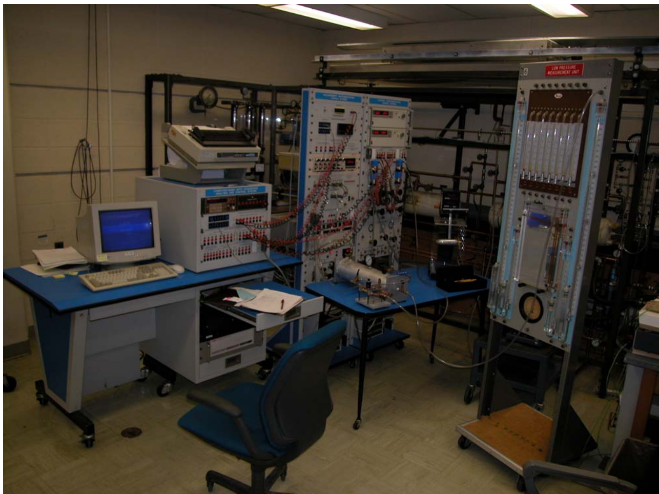
Figure 11: Computer Aided Data Acquisition Analysis and Control System (CADAACS)
