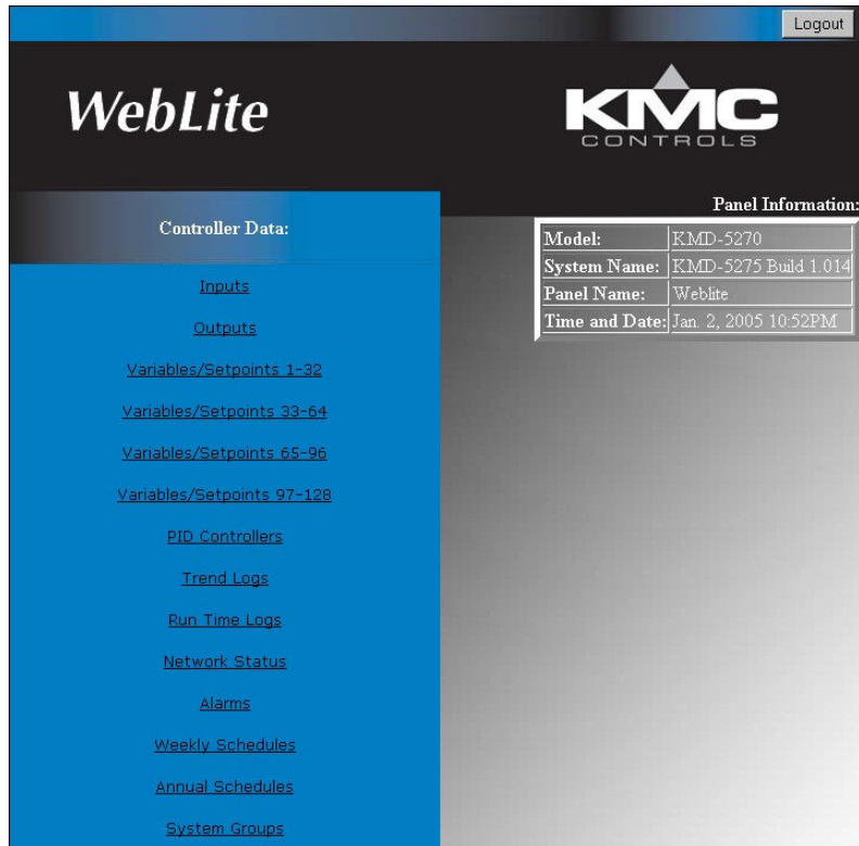
Figure 1. One web-enabled control system used for monitoring solar energy systems.
