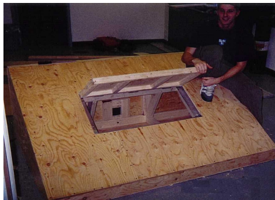
Figure 4. Hurricane roof vent test bed.
