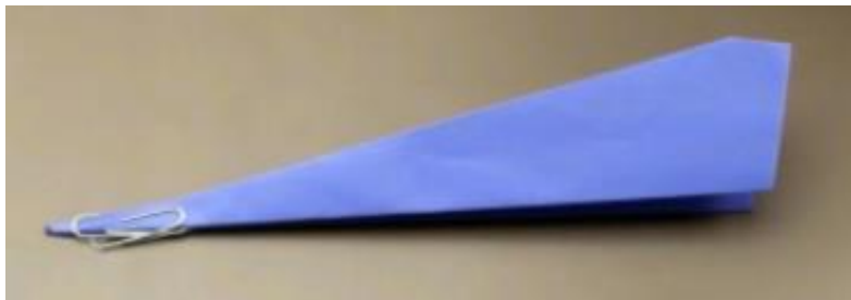
Figure 18 Paper Airplane with Paperclips Placed at Frontend
