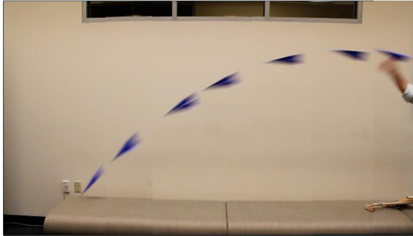
Figure 19 Video Snapshots of a Flight Path with Paperclips Placed on Nose
