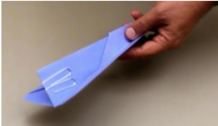
Figure 20 Paper Airplane with Paperclips at the Rear-end
