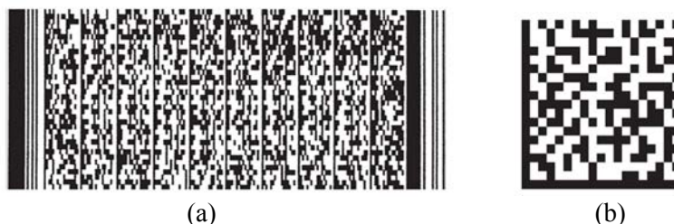
Figure 2: (a) 2-D stacked bar code and (b) 2-D Matrix barcode (Data Matrix)
