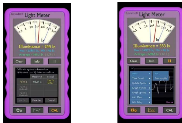
Figure 10: The installed application displays stored data (left) and the application displays graphing options and units (right)
