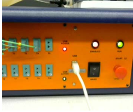
Figure 15: USB connection to heat exchanger
