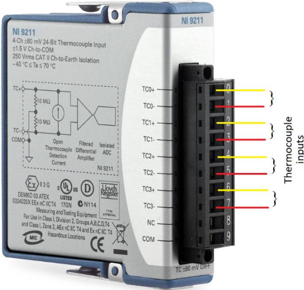
Figure 4. NI 9211 Thermocouple module used for data acquisition
