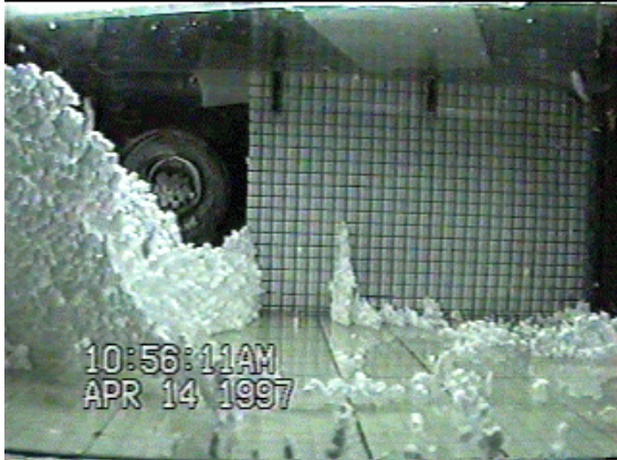
Figure 2: Styrofoam walls in microgravity: 110 mode, 1250 Hz. From Wanis et al, 1998 3 .
