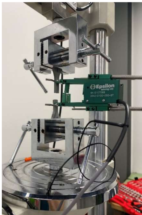
Figure 8 (a) Sample tensile test specimen (left), (b) Guide for test stand and extensometer (right).
