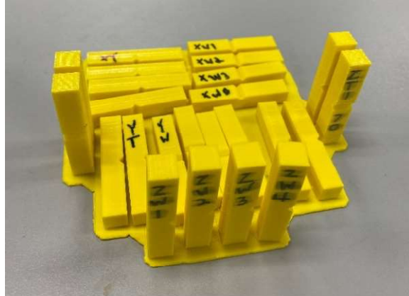
Figure 7 Charpy Specimen Orientation Coding (specimens printed along X, Y & Z axes).
